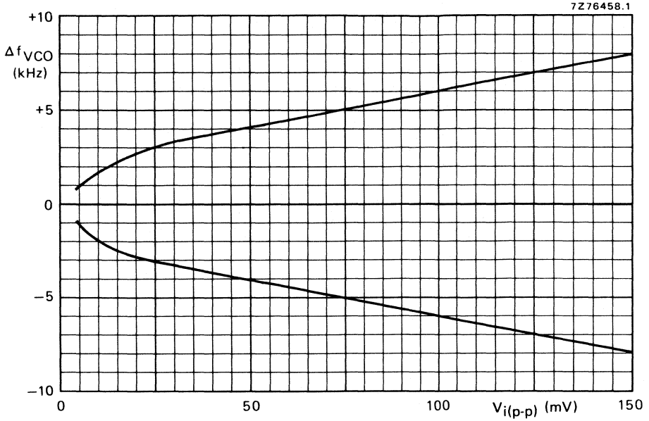
Fig. 27 Typical values of the capture range of the oscillator as a function of the pilot threshold voltage at MUX-input.
